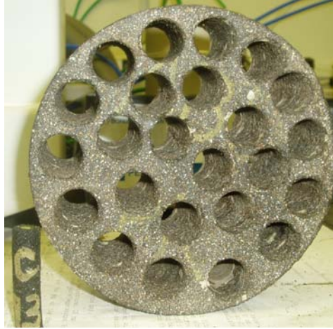
Figure 2. SGC Compacted Sample and 12 mm Sample for DMA Testing.
