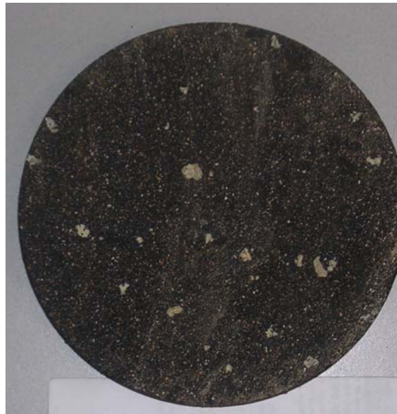
Figure 6. Type 3 Prills in AAD-Gravel Matrix.
